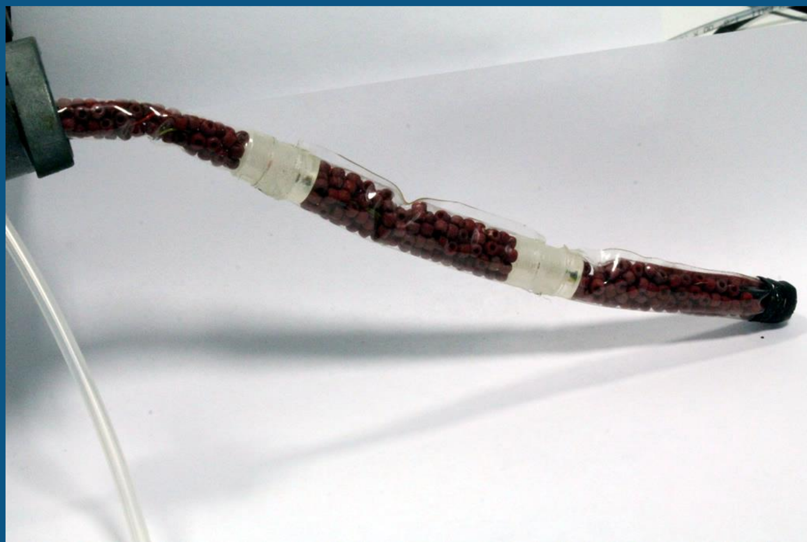
Figure 1. The Core-Snake, a granular jammed robotic limb for endoscopy. Current works on jamming have not examined the effect of coupling particles together, akin to connective tissue in animals. We present a study which provides a comparison between coupled and decoupled granules when jammed for a dexterous robotic limb.
